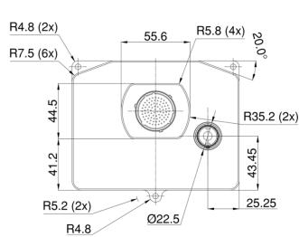
Note: Do not remove any part of the casing. The case provides electromagnetic screening to avoid interference with other equipment, and is also essential for thermal management. Thermal management may be compromised if mounted in a confined space, refer to the operating specifications.
