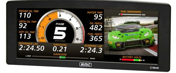
The C1812 comes standard as a combined 12" full colour display, powerful control device and fully programmable data logger with 250 MB internal memory. Optional USB Logging provides additional data capacity and flexibility, and also upgrades the internal memory to 500 MB.
