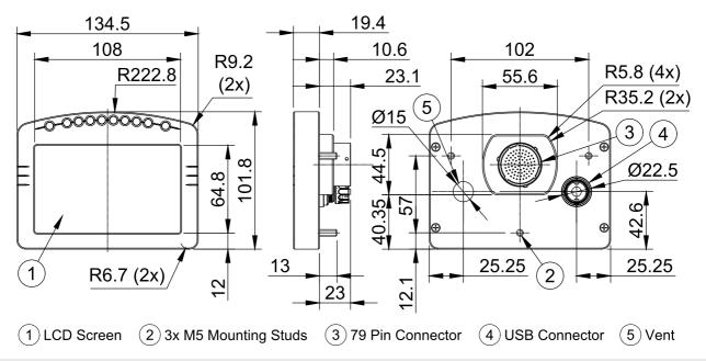
Note: Do not remove any part of the casing. The case provides electromagnetic screening to avoid interference with other equipment, and is also essential for thermal management. Thermal management may be compromised if mounted in a confined space, refer to the operating temperature specifications. Ensure product is not stressed when mounted.
