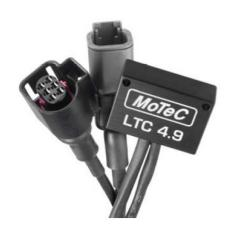
MoTeC's LTC (Lambda To CAN) monitors, controls and diagnoses a Bosch LSU 4.9 Lambda sensor, transmitting Lambda readings on a CAN bus. When using multiple LTCs, up to 32 Lambda sensors can be configured on a single CAN bus for simultaneous monitoring by an ECU or logging device.
