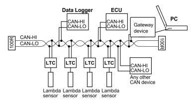
For information on wiring a CAN bus with several LTCs and any number of other CAN devices (as per the example), refer to the relevant device manual.
