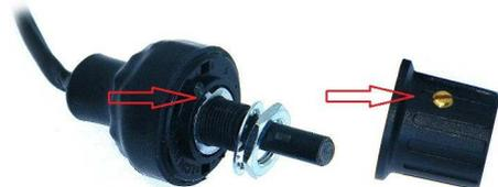
Beneath the M10 screw nut there is a dog ring to setup mechanically the maximum number of rotary positions. The dog has to be inserted according to the engraved number as the rotary switch shall have mechanical positions. It is recommended to secure the ring with a drop of silicone or glue prior to final mounting.
