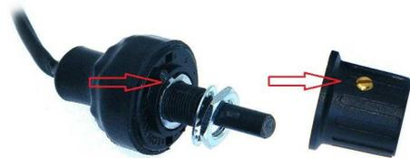
Beneath the M10 screw nut there is a dog ring to setup mechanically the maximum number of rotary positions. The dog has to be inserted according to the engraved number as the rotary switch shall have mechanical positions. It is recommended to secure the ring with a drop of silicone or glue prior to final mounting.
