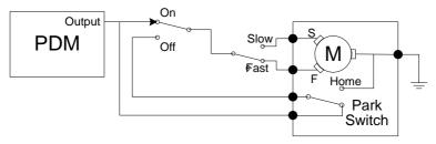
The wiper unit can be wired in a simple two switch arrangement; one switch for power and the other to select fast or slow. The PDM supplies power only.
